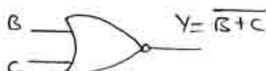
NOR  $Y = \overline{B}\overline{C} = \overline{B+C}$
